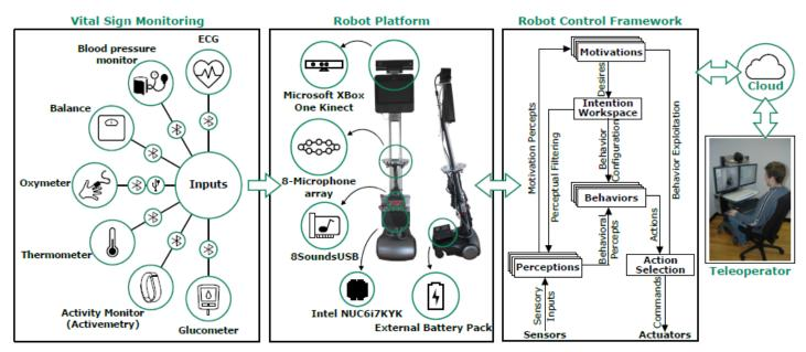
Figure 1: Enhancing a beam+ Telepresence Robot for Remote Home Care Applications
