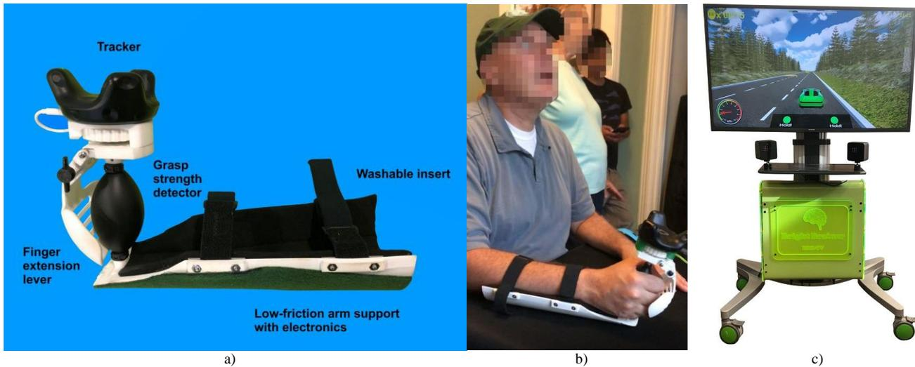
Fig 1. Telerehabilitation setup: a) BBG therapeutic controller [10]; b) Case 2 training at home while resting his affected arm on a low-friction mat; c) the BrightBrainer System © Bright Cloud International. Reprinted by Permission.
