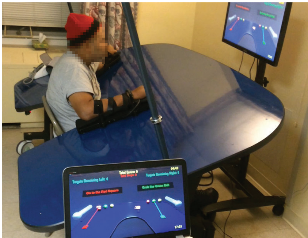
FIG. 1. BrightArm Duo system with a participant training at the “Pick & Place” game when the work surface is tilted upward. 18 ©Bright Cloud International Corp. Reprinted by permission. (Color images available at www.liebertonline.com/g4h )
